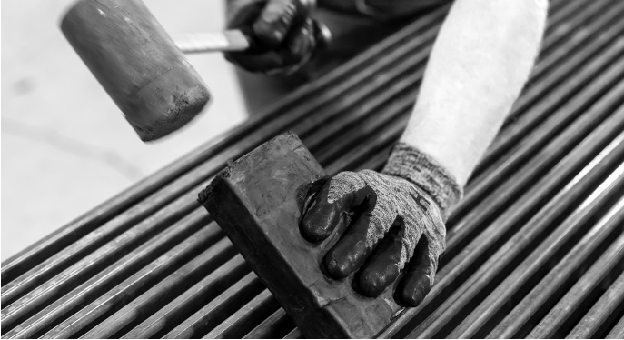
FIG.24 Straightening tubes with a wooden block & mallet
