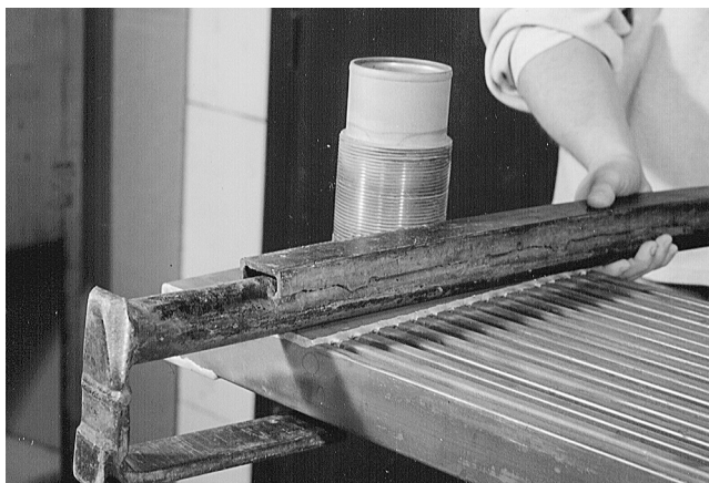
FIG.22 Locate twisting hook as close as possible to the nozzle or stud
